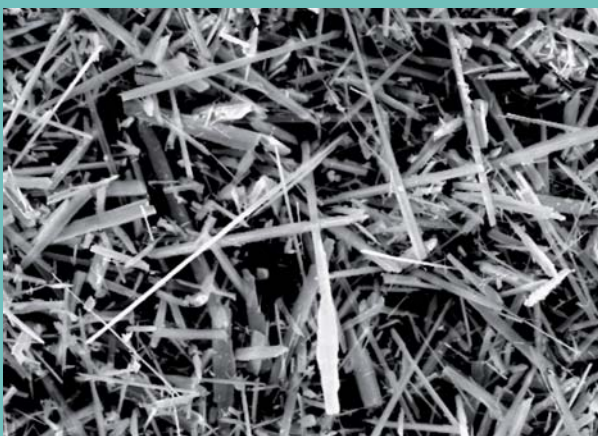
Microscopic picture from acicular wollastonite powder
