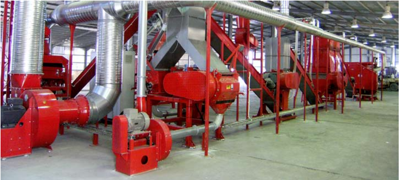
FIREFOX TURBO B – Chopping Line with Twin Granulator, Single Granulator, Storage Bin and Rough Chopper
