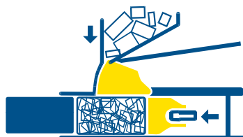
Main ram compresses with maximum pressure. Feed from conveyor to hopper above prepress resumed.
