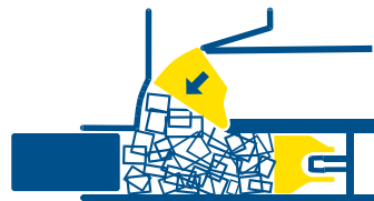
Prepress forces material into press chamber.
