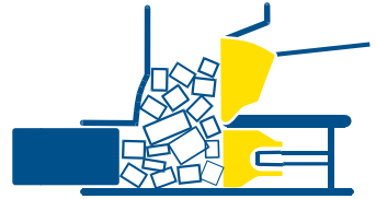
Prepress and main press in their starting positions. Press chamber full.
