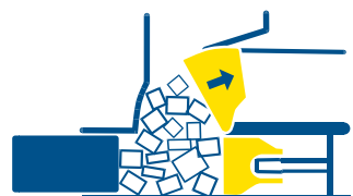
Prepress opens and material in hopper falls into press chamber.
