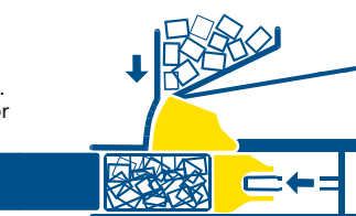
Main ram compresses with maximum pressure. Feed from conveyor to hopper above prepress resumed.
