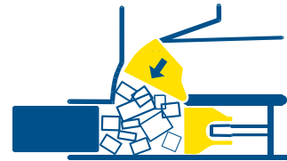
Prepress forces material into press chamber.
