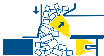
Prepress opens and material in hopper falls into press chamber.
