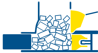
Prepress and main press in their starting positions. Press chamber full.
