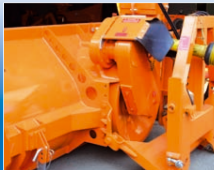
Chain gear with automatic tensioning device
