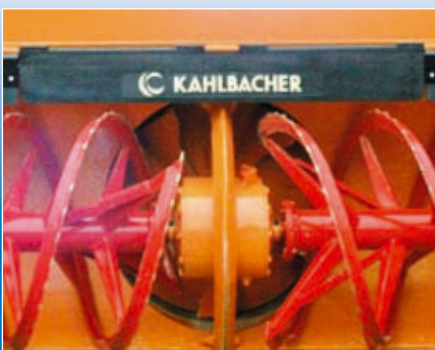
Front part of the snow-blower with augers and, located behind it, the impeller with large intakes
