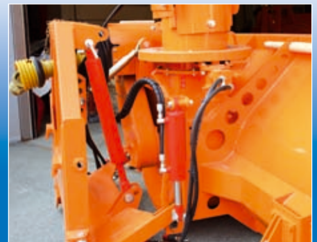
Hydraulically adjustable transverse tilting gear
