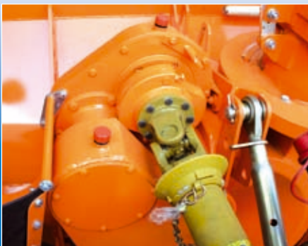
Impeller protected against overload by shearing pin clutch
