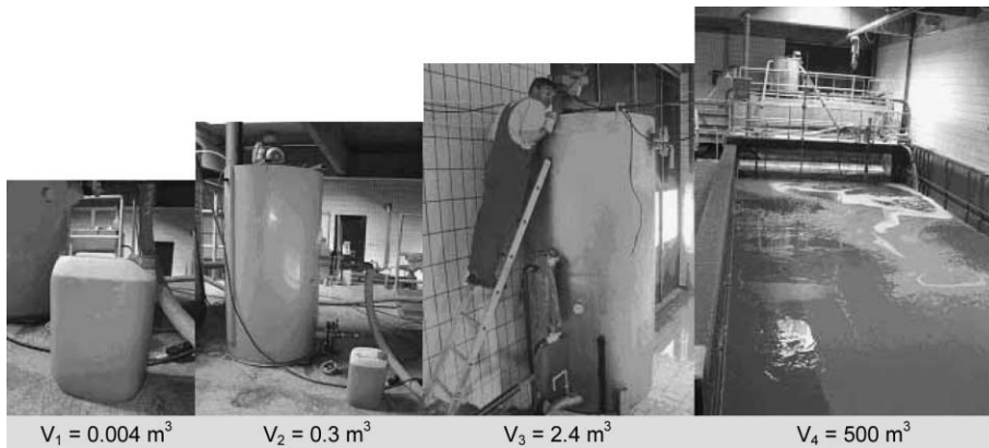
Figure 1 Gradual reactor size scale-up for enrichment of anaerobic ammonia oxidising biomass starting from 4 L of inoculum to the final reactor volume of 500 m 3
