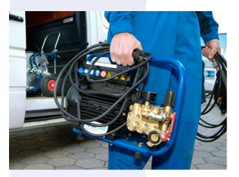
The MiniJet is a professional high pressure jetting machine, that can be taken everywhere without problems. It is suitable to clean drains from 25 – 100 mm.
