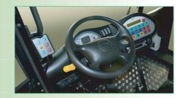
The Minor also features Scarab's tried and tested CANbus 2 control system, to give improved selfdiagnostics and additional compatibility with the J1939 CAN system to facilitate engine control and communication.
