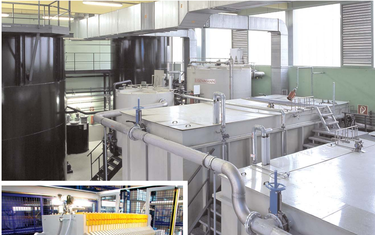
Purification of laundry waste water by flotation
