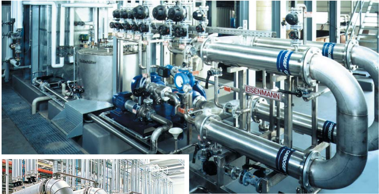
Top: Ultrafiltration system for emulsion splitting at a liquid waste disposal company.
