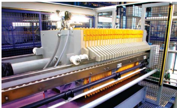
Chamber filter press for filtering of slurry
