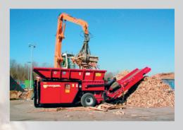
In addition to the stationary version, completely mobile and semi-mobile hook-lift versions are also available, to allow speedy relocation of the complete plant. The machines can be driven by either diesel engine or electric motor. The throughput performance of the complete processing plant is between 25 - 40 t/h\* depending on the end product
