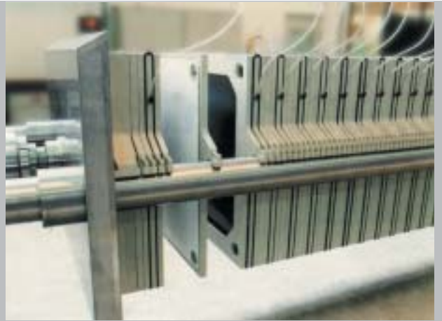
Filter press with filter plate combination for blood plasma filtration
