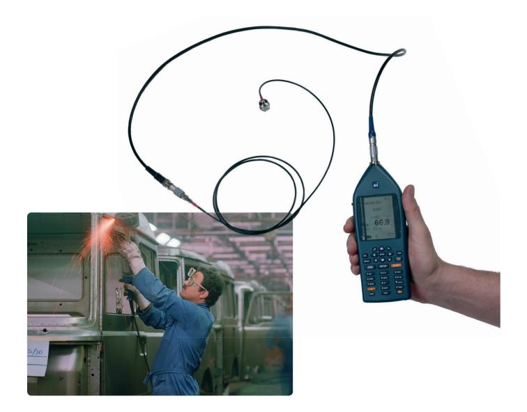
This technical note describes the use of the sound level meter Nor140 for measurement of acceleration levels. The normal microphone is then substituted by an accelerometer. The note also describes calibration and the relation between the level in decibel and the acceleration in linear units.
