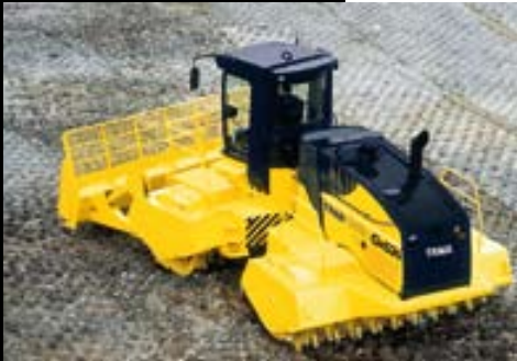
TANA TRC Construction (Twin Drums, Rigid Frame, Crushing Teeth)
