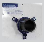
In case of fire, the Curaflam® collar XS shuts off completely flammable pipes with a maximum outer diameter of 200 mm. The collar will be fixed on both sides of a wall or underneath the ceiling and can also be placed around pipes in 45° position.
