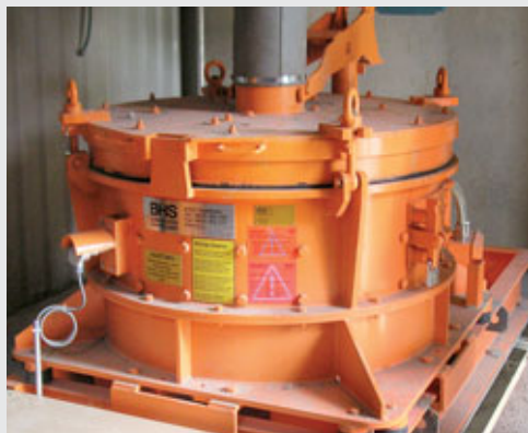
RPM 1113 for the production of concrete sand (0-2 mm) from gravel (16-32 mm)
