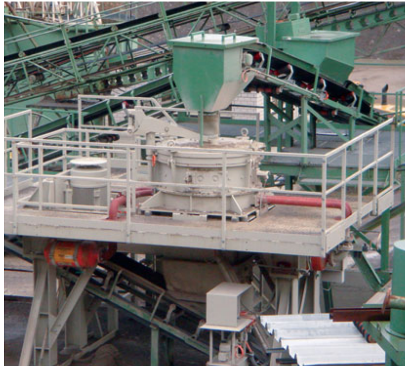
RPM 1113 for the production of concrete sand from limestone
