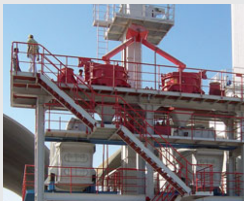
Two RPM 1513 for the production of dry mortar sand (0-1.6 mm) from limestone (8-20 mm)
