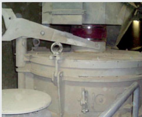
RPM 1113 for grinding of burnt lime
