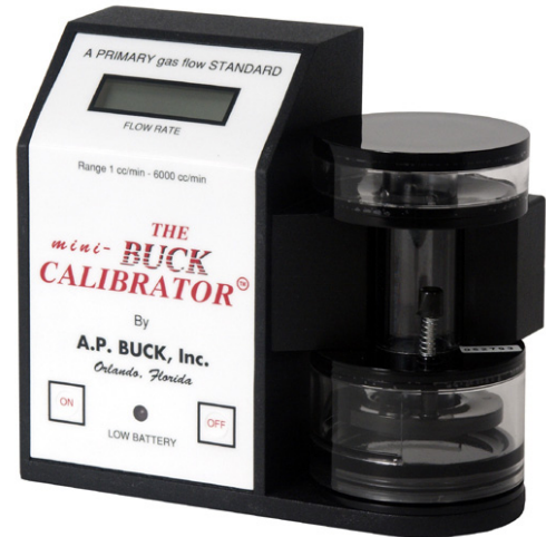
The first electronic gas flow standard, NIST traceable with accuracy of \pm 0.5\%
