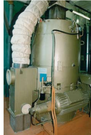
Pelleting press in a compound feed factory
