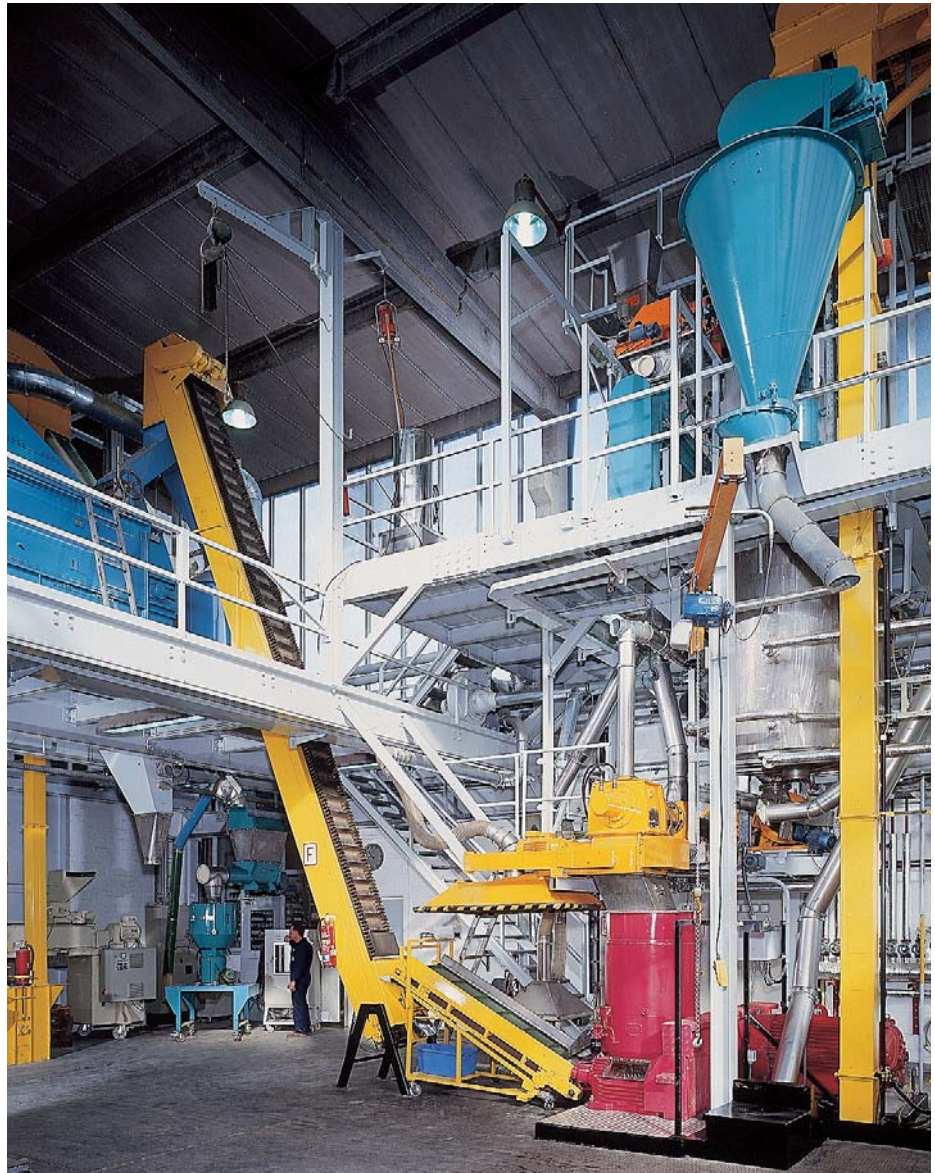
Pilot plant with proportioning unit, continuous mixer, hydrothermal reactor, annular gap expander, extruder OEE, flat die pelleting press, belt drier/cooler, Rotospray, crumbler
