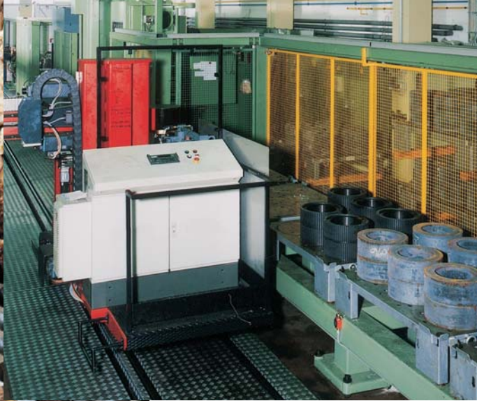
Production line for pan grinder rollers using a robot-shuttle
