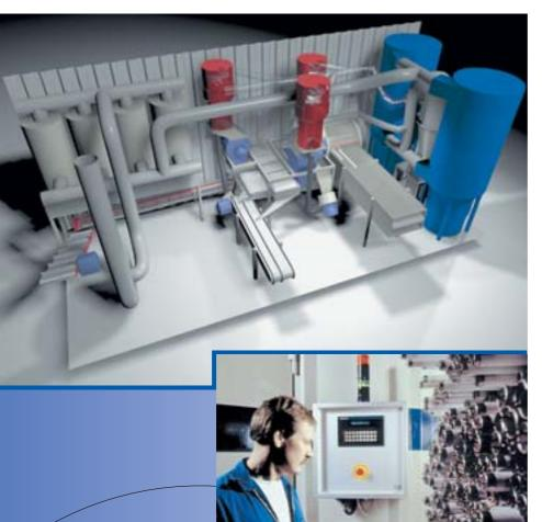
◀ The entire process is incorporated in a container, in which the air is brought to sub-pressure. Thereby preventing mercury from being released into the environment, as exhaust air is constantly discharged through the internal carbon filters.
