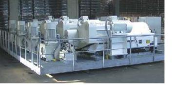
**HILLER®** decanters have been used for 'drilling mud' in vertical exploration drilling for the development of oil and gas fields for more than 20 years.
