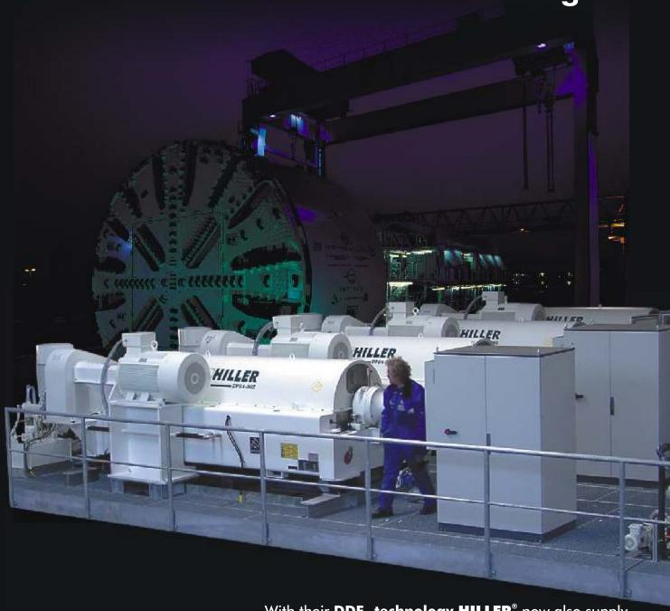
With their **DDF** technology **HILLER**® now also supply high-grade dewatering decanters for substantially larger tonnages of accumulating drilling mud at a continuously high dewatering performance level.
